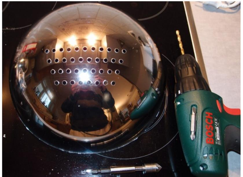
I used a spanner and 2 wires to force a egg shape. wires go through the 2 extra holes which are below the ones for the elastic. adjust as you want it. Force it a little bit more because after tempering it will spring back a bit.
